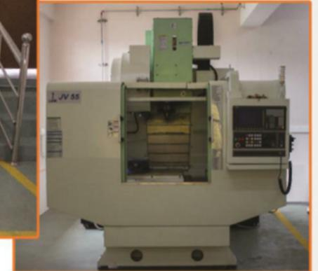
SINUMERIK 808D control is a panel-based CNC for the basic performance range. It is used for basic turning and milling applications. Sequences can be programmed and simulated offline. Different type of cycles can be used to perform machining operation using 808D Controller. SINUMERIK 828D Controller is the advanced version of 808D controller. The advantage of this controller is that it is possible to simulate the operations prior to actual machining.
